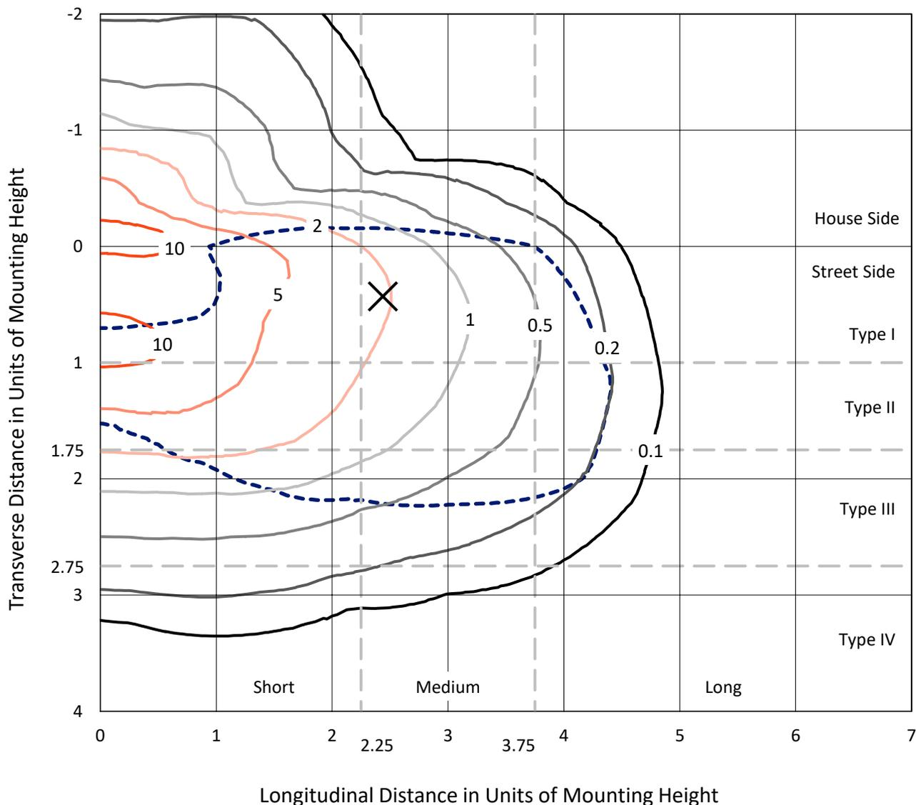
Based on 20 foot mounting height. Maximum calculated value = 12.5 fc
